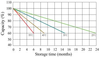
Temperature effects on capacity at 0.5C
