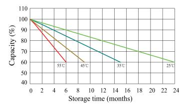
Temperature effects on capacity at 0.5C
